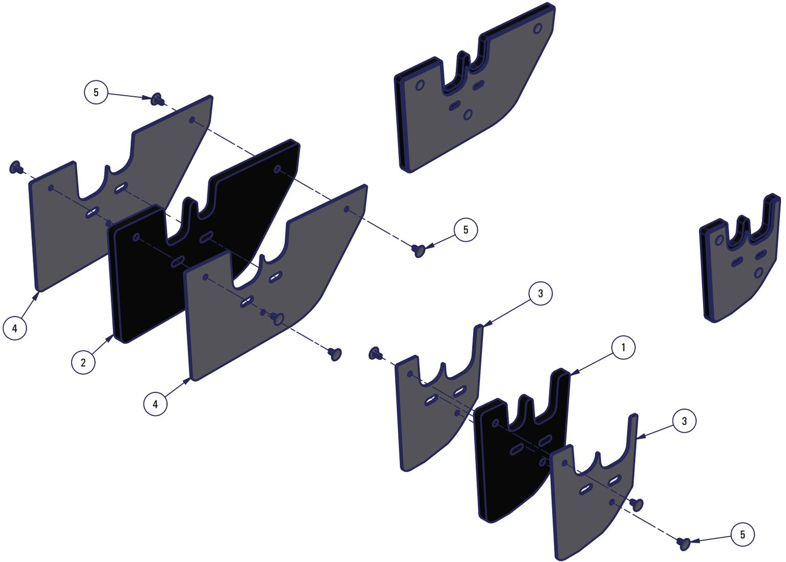
Step 1: Use the provided hardware to assemble the gun rack \ dividers. Place a stiffener on each side of the foam and line up the holes.
